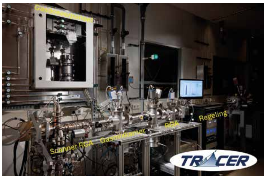
Figuur 10. TRACER-opstelling TNO: Tool for RGA Accuracy and Calibration Enhancement Research. (Foto: TNO / Jurjen Poeles)
